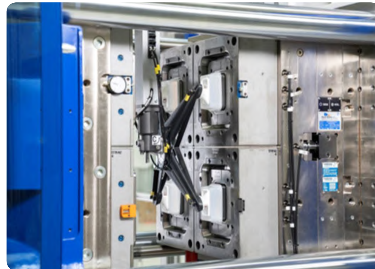
EcoPower Xpress 300/1100+ – demolding of margarine tub (Foto: WITTMANN BATTENFELDI)
