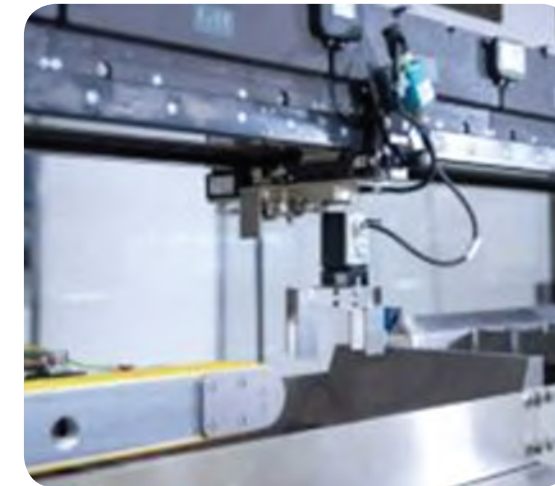
The grippers move independently of each other and operate at top speeds (Image: Rotzinger)
